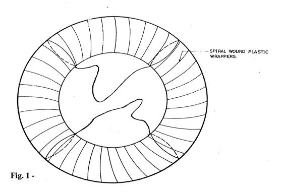
SLING ARRANGEMENT FOR LIFTING 63 mm \$\phi\$ COILS
