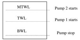
A Series of float switches or any other PLC system shall be used to monitor the level of fluid in the sump and the control system shall be monitors these float switches and determines which pump is to be started. The pump operating system shall be as follows.
